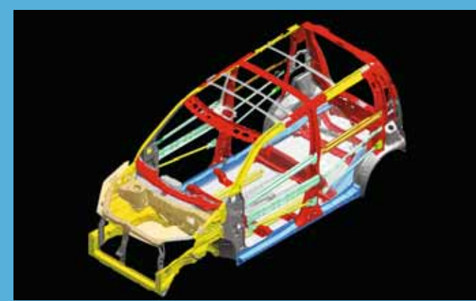
Energy absorbing body structure for safer drives
